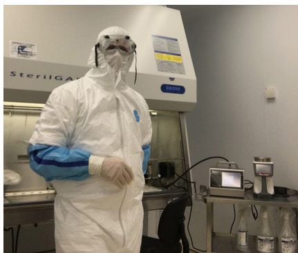
Figure 1. Operator testing air quality in the ISO 5 Biological Safety Cabinet
