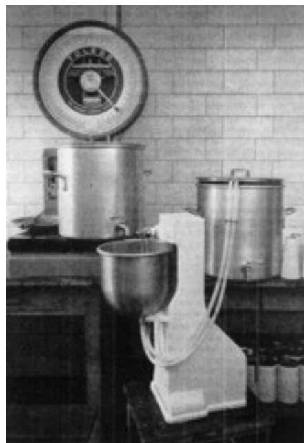
Equipment used for homogenization of formula in 40-kg batches
